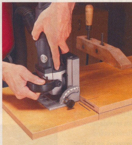
B Stand your plate joiner on end to cut slots in the side of the case. The end of the shelf is a built-in straightedge.
