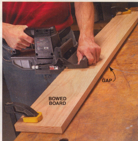
Reduce sanding time by aligning bowed boards with biscuits. Reference your plate joiner fence from the top of each board.
