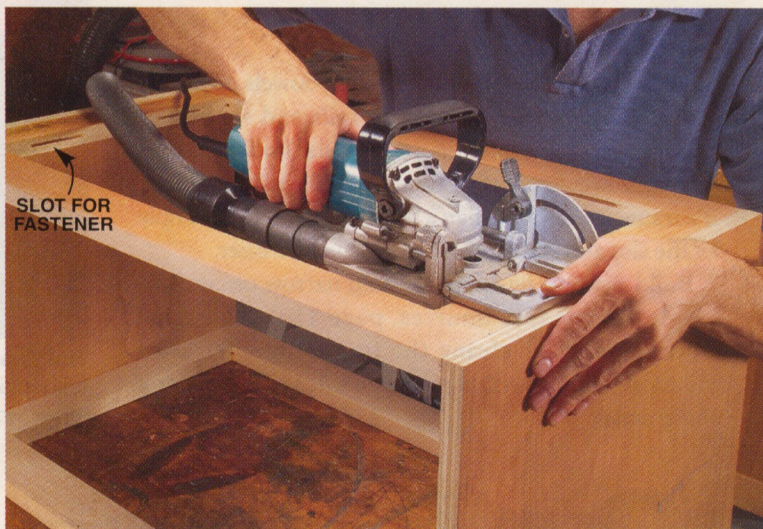
Use your plate joiner to cut slots for tabletop mounting clamps.
