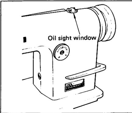
As long as the oil reservoir is properly filled up with the lubricating oil, you will see the oil splashing on the internal surface of the oil sight window while the machine is running. Since the oil sight window is used only to check if the lubricating oil is flowing or not, you do not have to worry about the amount of oil appearing in it.
